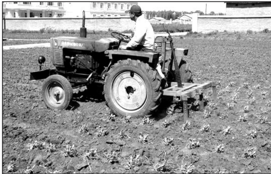
The typical tractor we saw in Heilongjiang was powered by a one cylinder diesel engine mounted on two I-beams. In early June, they were being used to cultivate between the crop rows. Photos by Daryll E. Ray
